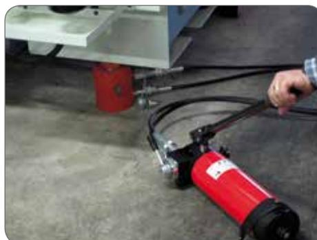
*PDSA20 DE pump to operate a double-acting cylinder to level large machinery.*
