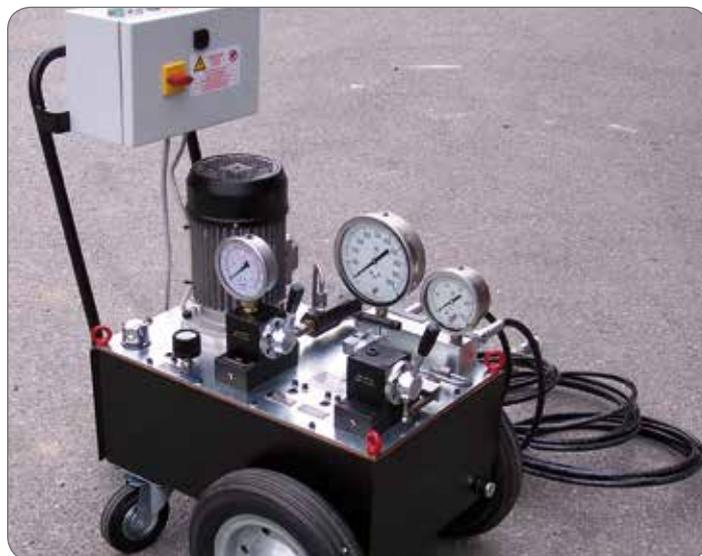
*Hydraulic pump to operate strand jacks in the field of post-tensioning*
