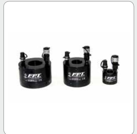
Hydraulic nuts series operating pressure 2,250 bar for tension rods M36 - M56 - M72 with treated surface and special coatings for environments with high working temperatures. Hydraulic nuts can be made to the customer's specifications to get the most out of the clearances available.
