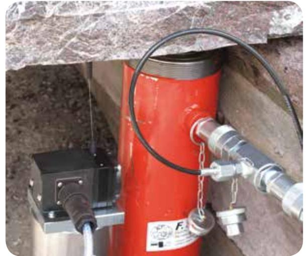
Wire transducers to control the stroke
