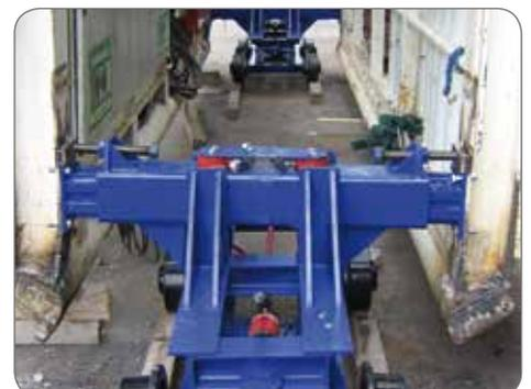
Equipment to support decks in tunnels consisting of a PMSA 3.5 pump and 10-ton cylinders.
