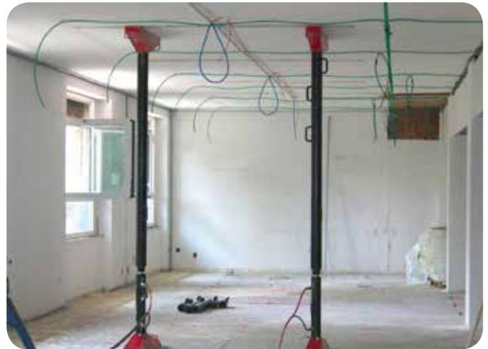
Hydraulic kit for floor Load Tests, used to carry out static load tests with concentrated load. Kit comprising support cross members, hydraulic cylinder, light alloy extensions and hydraulic pump
