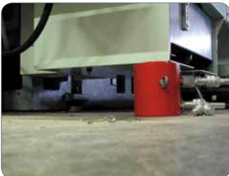
50-ton CRIC for lifting mechanical workshop machinery.
