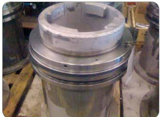
Hydraulic nut for propeller shaft-rudder coupling.
