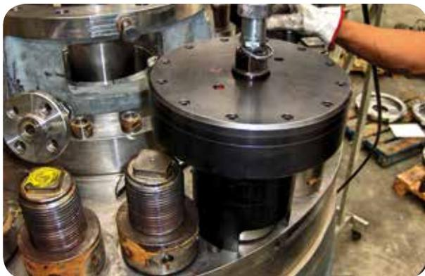
M64x4 120-ton capacity hydraulic tensioner with spring to return the piston.
