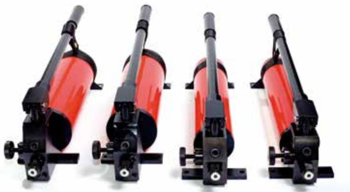
The PMS and PDS pumps have been specifically designed to operate hydraulic tensioners. Available in single- and two-speed for pressure from 1.600 to 2.800 bar.
