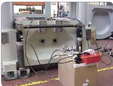
*Pump with 8-litre reservoir for lifting a press section.*
