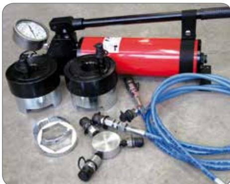
Complete set for very high pressure pump to operate tensioning devices.
