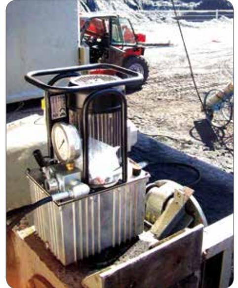
Electric control unit for lifting a roupelle.
