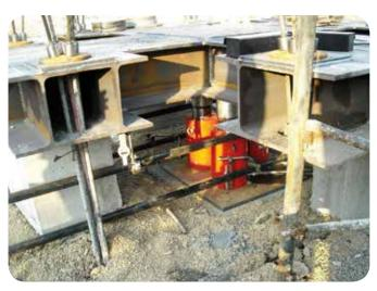
Load tests on foundation piles and failure recording with 250 ton-capacity, 250 mm stroke F.P.T. cylinders - model CRI250/250
