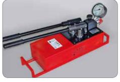
Pump for hydraulic stud bolt tensioning equipment for marine engines.
