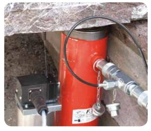
Wire transducers to control the stroke
