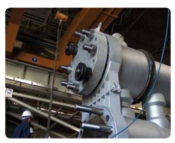
HYDRAULIC TENSIONERS FOR BOLTING HEAT EXCHANGERS
