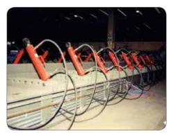
Systems for hot forming large support piles using 22-ton CDE cylinders with Viton gaskets to withstand high temperatures.
