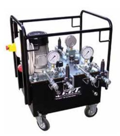
Hydraulic pump with 4 independent delivery ports with single overcentre valves (700 bar) to synchronise the load in both lifting and lowering.
