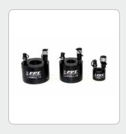
Hydraulic nuts series operating pressure 2,250 bar for tension rods M36 - M56 - M72 with treated surface and special coatings for environments with high working temperatures. Hydraulic nuts can be made to the customer's specifications to get the most out of the clearances available.
