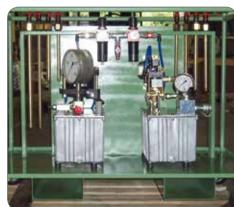
Unkeying unit with double pneumohydraulic unit (700 bar and 3000 bar).
