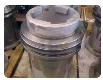
Hydraulic nut for propeller shaft-rudder coupling.
