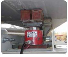
100 ton-capacity compact cylinder - Model F.P.T. CRM100/50C 100 ton capacity, 50 mm stroke
