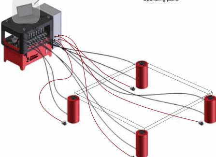
Typical layout for synchronous system from 4 to 8 points:
