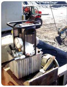
Electric control unit for lifting a roupelle.
