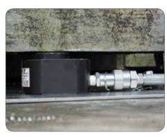
CRM 30/10 XP used to align machinery.
