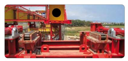
CDE 25/1650 (25 ton, stroke 1650 mm) double-acting cylinder, basculating with plate and pins.
